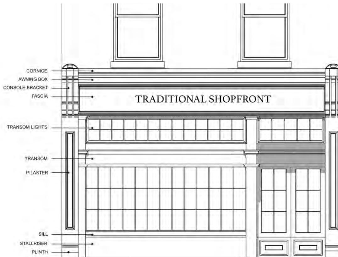
Figure 1 Key components of a traditional shopfront
