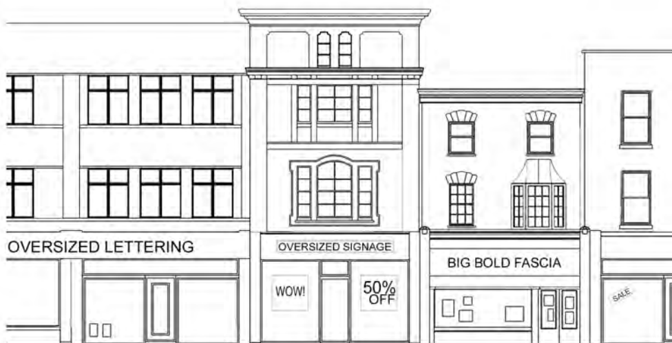
Figure 4 Shopfronts that have little or no cohesion with inappropriate alterations
